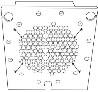
\*Four fixed tubes (cannot be removed) identified by adjacent drill points.
